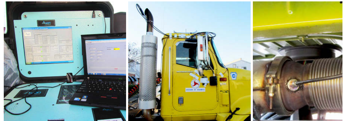
(Left) Portable emissions measurement system instrumentation in truck cab. ▶ (Middle) Truck instrumented to measure emissions during driving. ▶ (Right) NO x concentration sensor next to selective catalytic reduction reactor.
