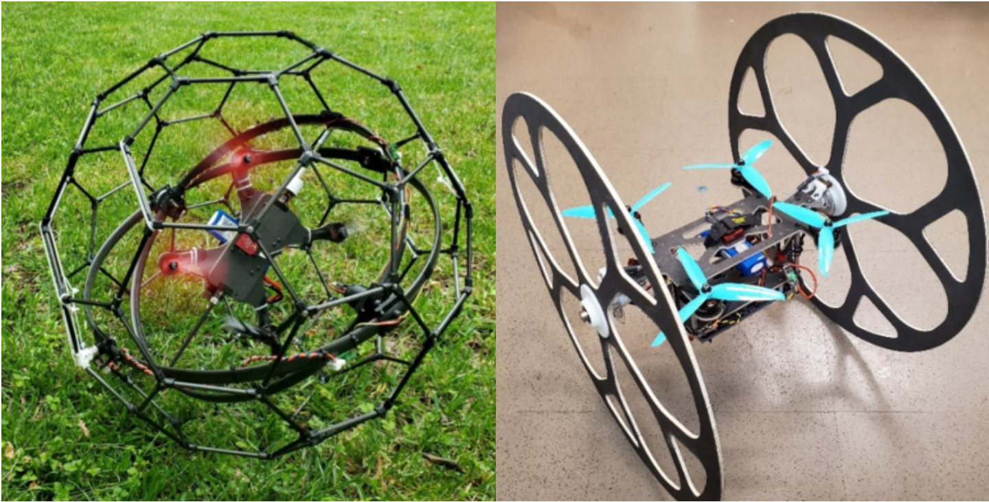
Figure 1: Two RFVs. While on the ground the rotors provide thrust, steering, and orientation control while the cage/wheels are passively towed. (left) The spherical RFV (SRFV). A spherical carbon fiber cage permits rolling locomotion and provides protection. The 3-axis gimbal system decouples the quadrotor from the cage, permitting omnidirectional rolling while reducing sensitivity to disturbances. (right) A two-wheeled RFV (WRFV).
