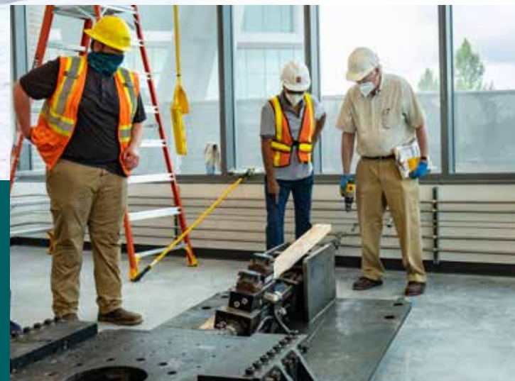
DRS. TASNIM HASSAN and DAVID JOHNSTON seen here instructing moving contractors exactly where to place the base for a shake table used in earthquake engineering research. The base weighs about 4,000 pounds, so placement in the right spot in the new laboratory is important.
