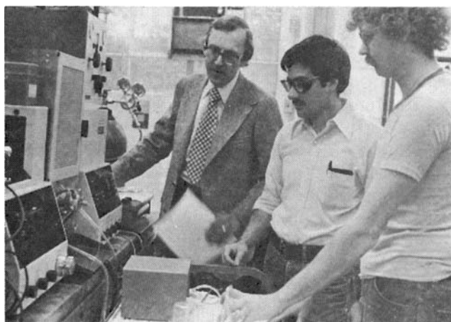
P Professor Ferrell, graduate student Victor Agreda, and laboratory technician Larry Hamel analyze a coal sample using an atomic absorption spectrophotometer.
