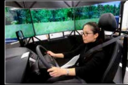
**ITRE AND THE DOT** are using the new simulator to model how drivers deal with certain road configurations and traffic signs and plan to use the data to help design roadways.
