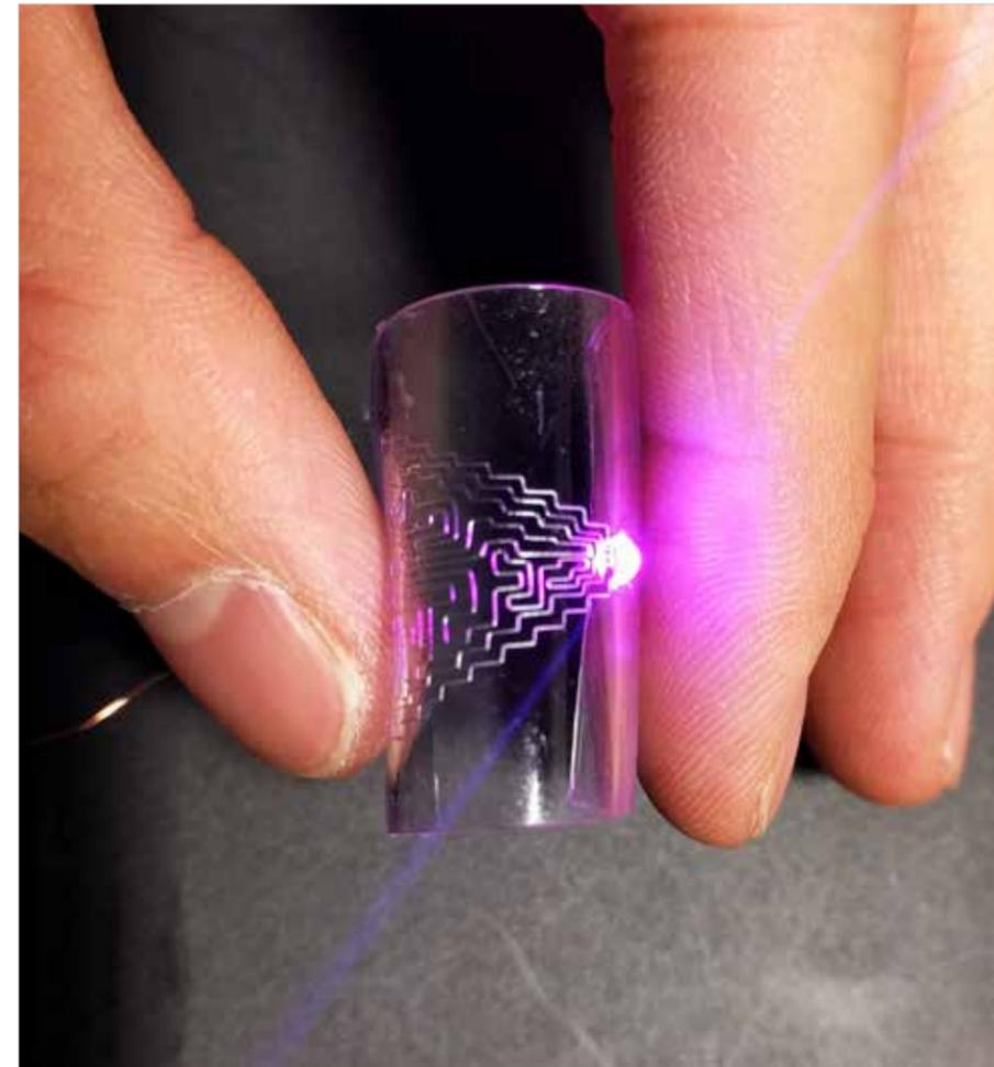
**RESEARCHERS IN THE COLLEGE** have developed a new technique for directly printing metal circuits, creating flexible, stretchable electronics. The technique can use multiple metals and substrates and is compatible with existing manufacturing systems that employ direct printing technologies.
