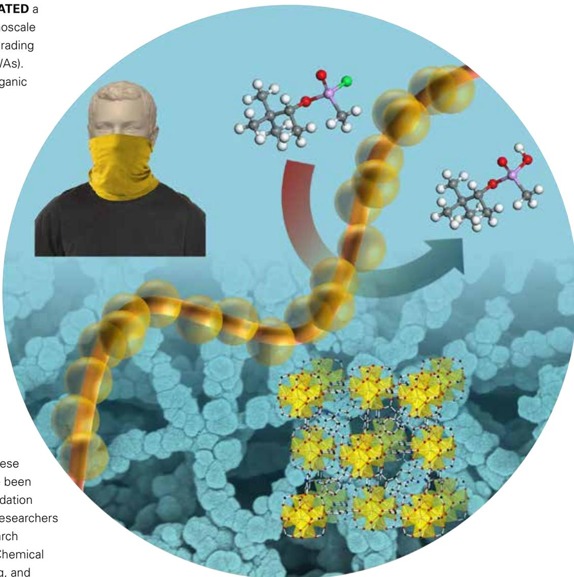
The researchers begin by depositing a thin film of titanium oxide onto a fabric made of nanoscale fibers using a vapor-phase technology called atomic layer deposition. The titanium oxide serves as a nucleation layer, which enables the researchers to apply various zirconium-based MOFs onto the nanofibers in an evenly distributed way.
