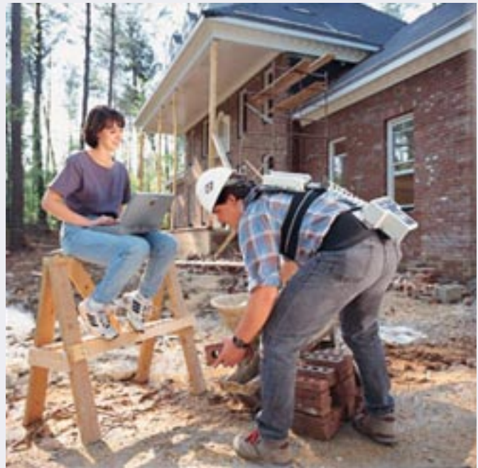
Two of Gary Mirka’s graduate students, Jennie Psihogios and Daniel Kelaher, illustrate the use of a Lumbar Motion Monitor at a construction site to quantify low back stress during construction work activity.
