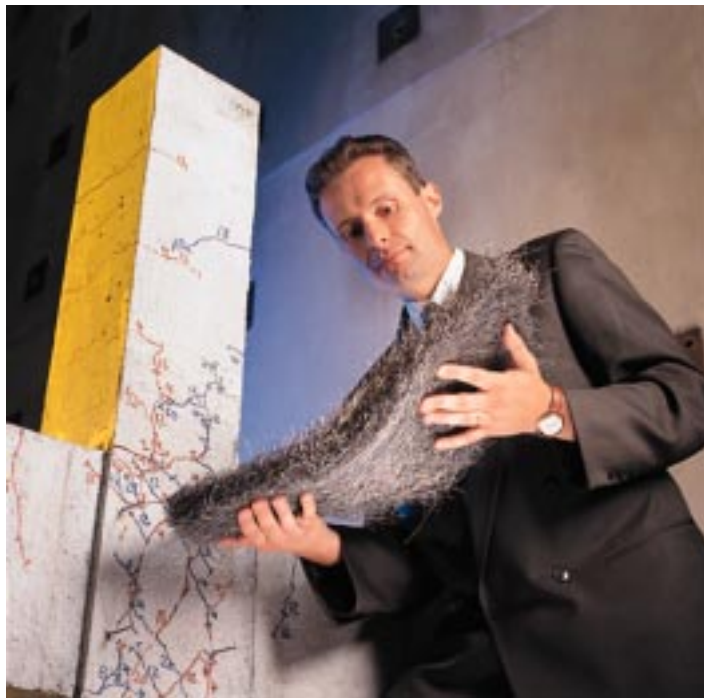
Neven Krstulovic-Opara holds a novel stainless steel fiber-mat used for manufacturing of Slurry Infiltrated Mat Concrete (SIMCON).
