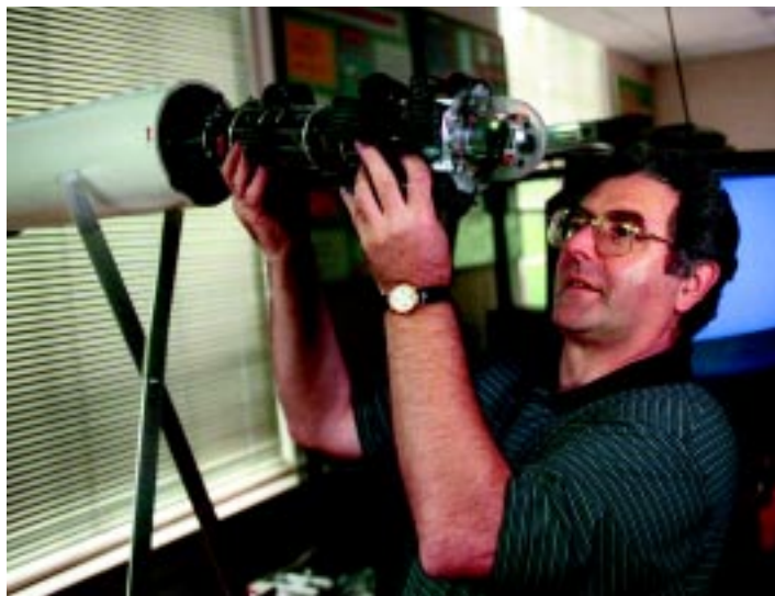
The pipe-crawling robot developed by students at NC State under the direction of Eddie Grant (pictured) and John Muth could help rescuers find survivors trapped in collapsed buildings.
