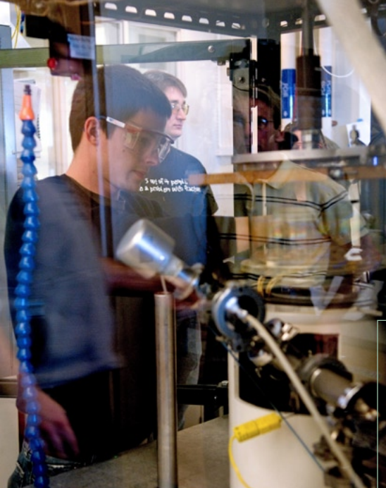
The atmospheric plasma chamber is key to the more efficient, cost-effective process developed by the team.
