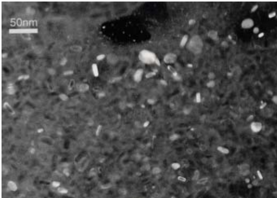
Fig. 8 Dark field transmission electron micrograph of nanostructured zinc.
